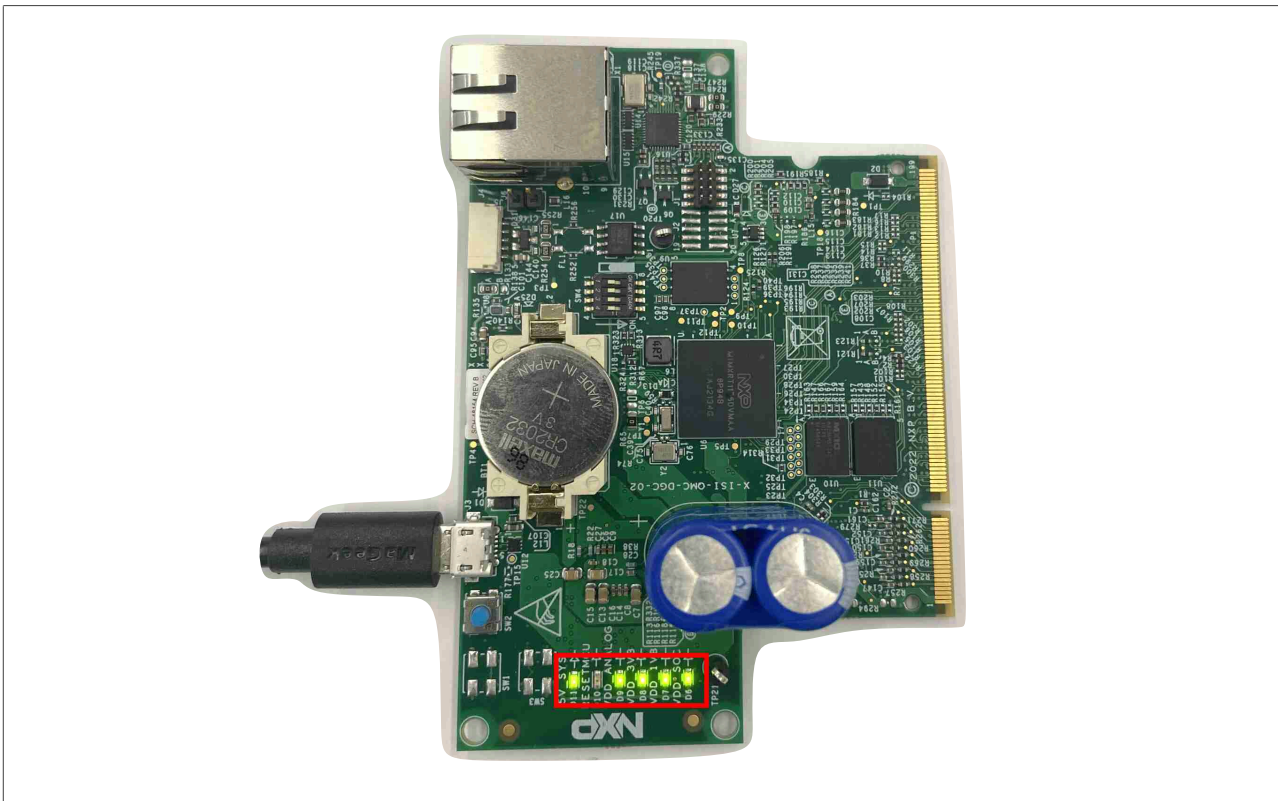
Figure 3. Daughter card supplied using the micro-USB connector (standalone operation)
